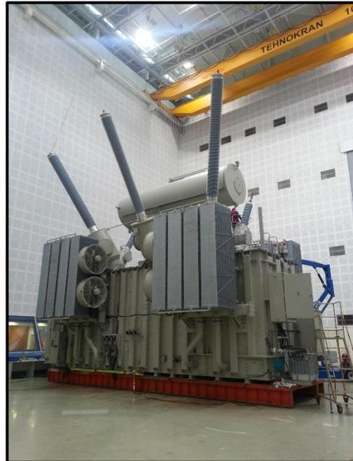
**Figure 3 Spare 2 during FAT with 420 kV bushings.**
