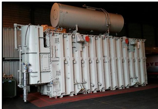
**Figure 4 Spare 1 with detachable OLTC and conservator on tank in warehouse.**
